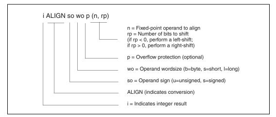
Figure 2-7. AutoCode/C Conversion Macros for Fixed-to-Integer Conversions
